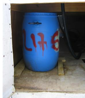
Photograph 2. 15-gallon drum with wooden guides.
