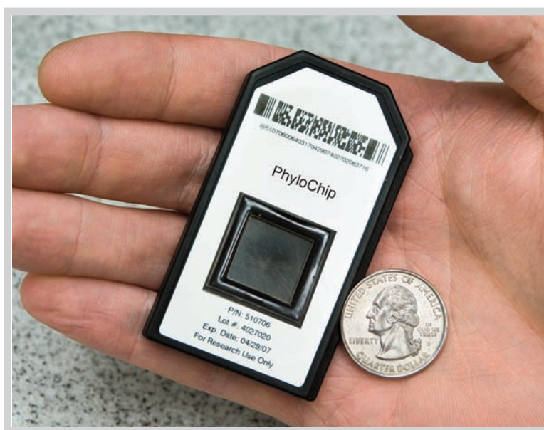
Figure 1. The Berkeley Lab PhyloChip profiles microbial populations at a rate and with an accuracy heretofore unknown. It simultaneously detects most known microorganisms (over 8,000 species tested in parallel) without culturing.
