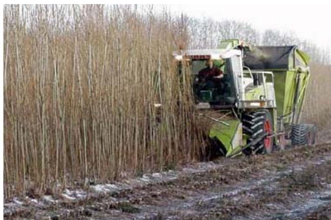
Figure 21: The willow (Salix) cuttings in the energy forest take only a few years to reach harvest maturity. They are cut and made into chips for burning as fuel. The trees do not need to be replanted, as new shoots will grow from the old root system.
