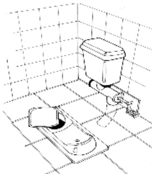
Figure 4.11 A mechanical, pedal-operated, ash dispenser used for school toilets in the Yongning eco-village programme (see 3.1.1 – China). (Design: Lin Jiang, 1999).
