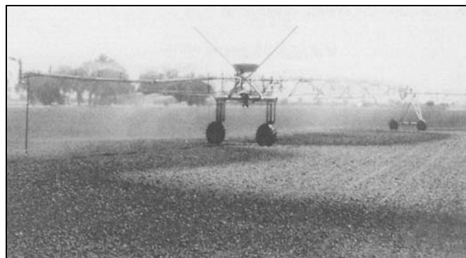
Figure 7-12 Center Pivot Sprinkler Unit.
