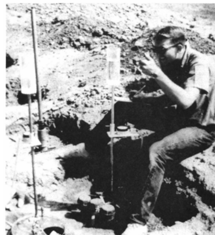
Figure 3-19. Air Entry Permeameter in Use (from H. Bouwer).
