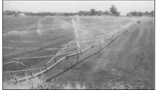
Figure 7-9. Side-Wheel Roll Sprinkler System.
