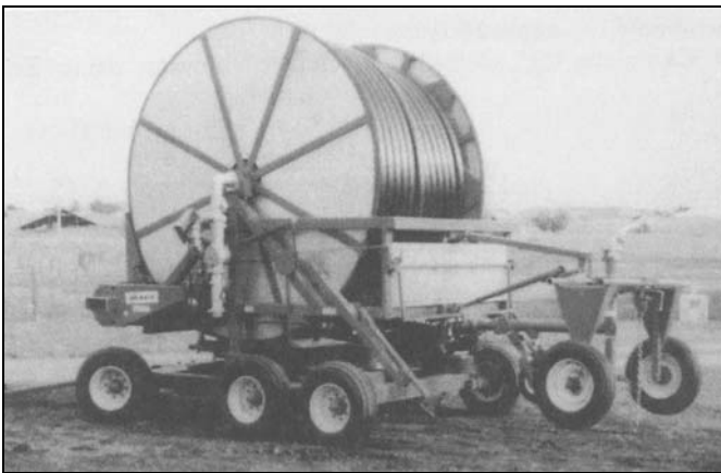
Figure 7-11. Reel-Type Traveling Gun Sprinkler.
