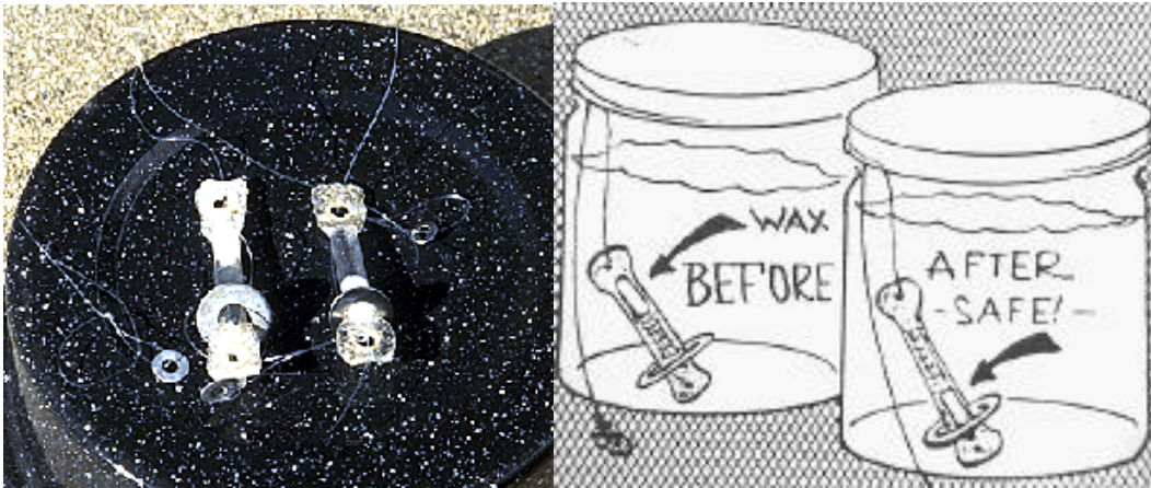
Figure 6: The WAPI is an invaluable tool that utilizes wax as a recording thermometer substitute.
