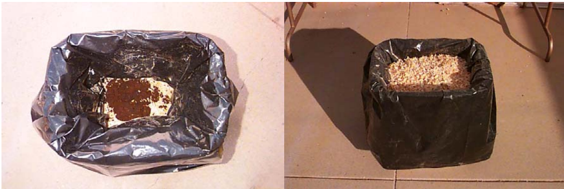
Figure 16: One week of waste collection (with urine diversion assumed) was simulated in these photos. The container is a standard 13 gallon kitchen trash can lined with a heavy duty black polyethylene bag and an autoclavable polypropylene bag. In early tests polyethylene bags were melting at folded spots.
