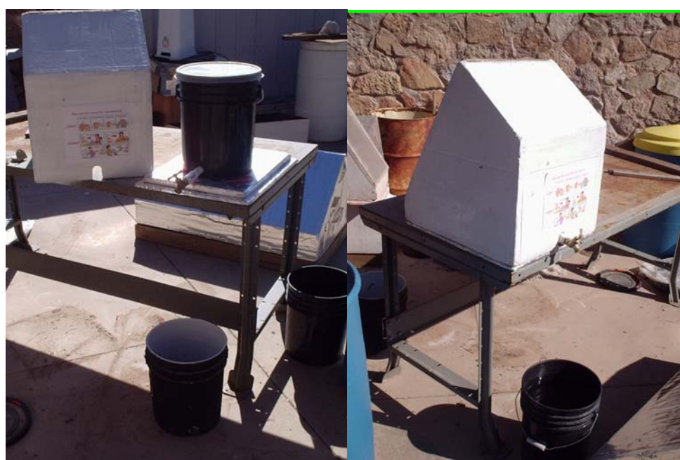
Figure 20: A glazed, insulated cover can extend the time of year for providing warm water. Caution should be used to prevent children from using water that may be too hot.
