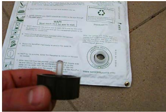
Figure 8: A WAPI type indicator is built into the Aqua Pak. When the wax melts and runs to the low end of the tube pasteurization temperature has been reached.
