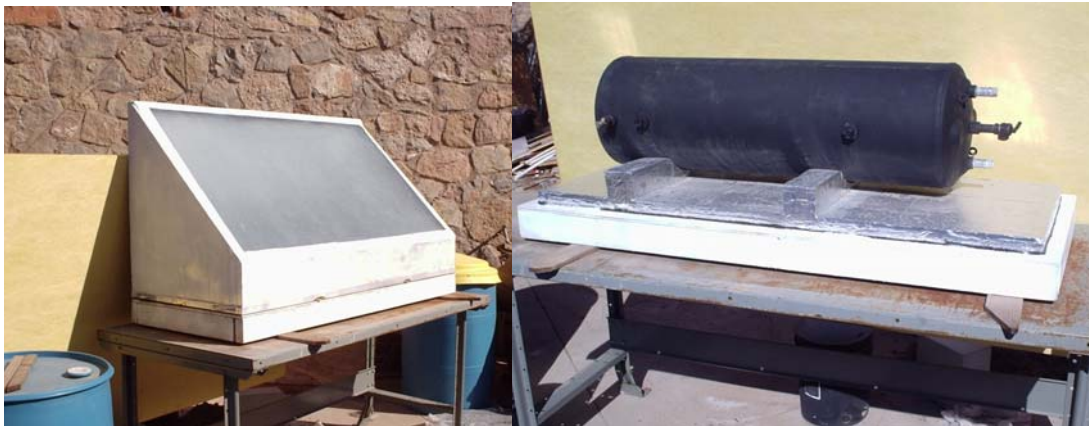
Figure 24: An old water heater tank can be converted into a passive solar water heater. In this design the weight is carried by a simple skid, allowing a lightweight insulated cover.
