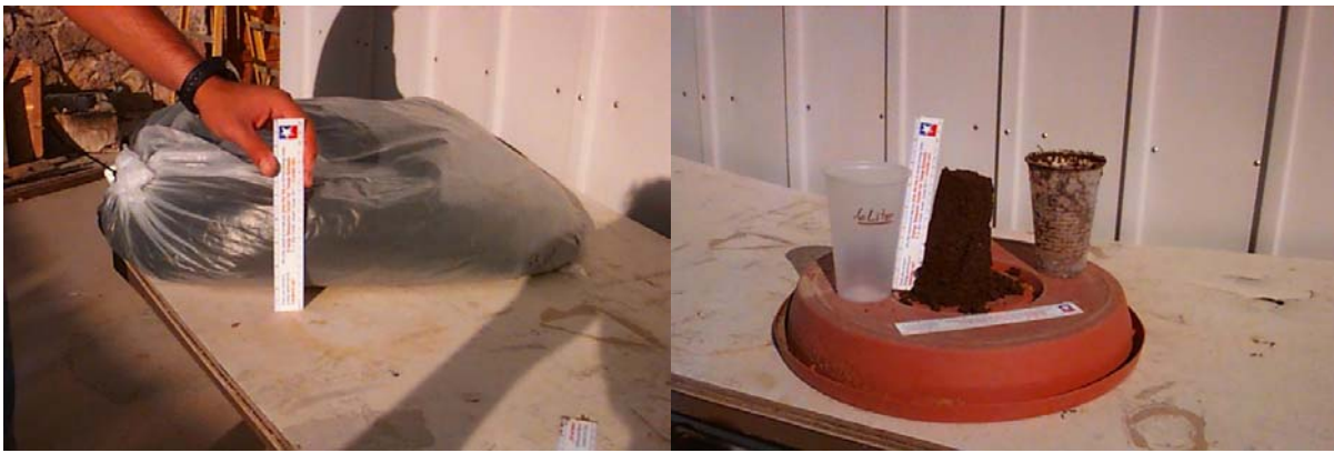
Figure 18: Bagging the waste also allows for a large surface area for solar collection to ensure a minimal and even depth for uniform heating for pasteurization. At right, .6 liters (20.3 oz.) of simulated solid waste (cow manure) is shown.
