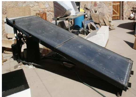
Figure 10: The Sol*Saver is large and expensive but has a high production rate and can operate automatically without any external power.
