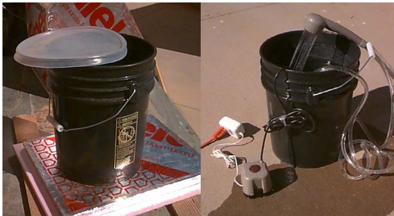
Figure 23: A black 5 gallon plastic bucket can provide hot water at a very low cost. A camping shower can be adapted to provide convenience if desired.
