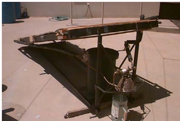
Figure 10: The Sol*Saver is large and expensive but has a high production rate and can operate automatically without any external power.
