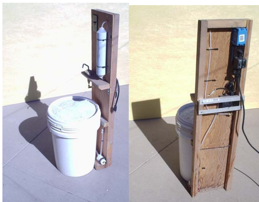
Figure 3: UV treatment is simple. Water is pumped through a cartridge exposing it to UV-C radiation and then out a faucet.
