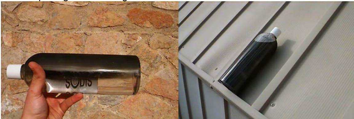
Figure 2: Solar disinfection of water is a simple and effective technology. Since there is no indicator or water safety the procedure must be carefully followed.
