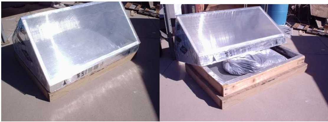
Figure 15: A later version of the pasteurizing unit features a 45 degree angle for the glazing to optimize for year round solar collection in El Paso (latitude + 15 degrees). The lightweight top simply lifts off the insulated base for loading and unloading.
